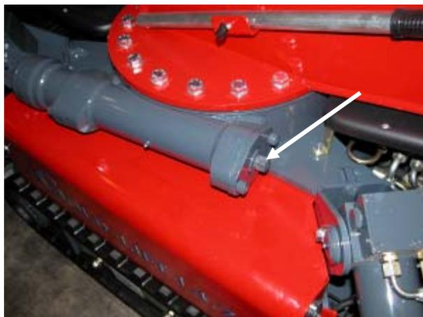
In the model 1470 when you are using the emergency descend, the jib cylinder cannot be activated; this means that when the arm is completely down, the basket is at about 1,8 m height. In this case, in order to help the person in the basket, it is necessary to use an external tool (for example a ladder).
