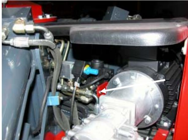
1. energize the mechanical activation of the electrovalve, pushing and turning the golden knob near the electrovalve coil.
