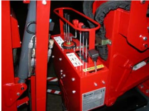
Both the translation and the stabilization are possible only if the machine is closed and aligned.
