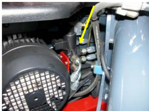
With the deviator you choose to convey the oil to the valveblock either of the undercarriage part or of the aerial part. If the coil is not energized, the delivery A is conveyed to the aerial part, the delivery B is conveyed to the tank. The aerial part uses only one pump. This condition happens when the machine IS NOT ALIGNED. On the contrary, if the machine is ALIGNED, the deviator is excited and the oil is conveyed to the undercarriage part.
