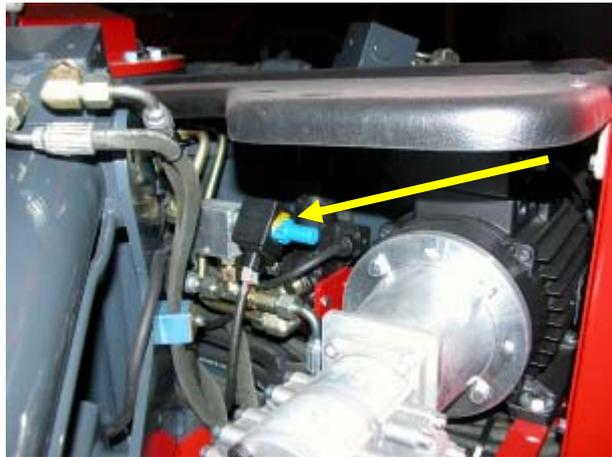
If this electrovalve is NOT POWERED, the oil is conveyed to the tank, preventing the movement of the aerial part. This condition happens when:
