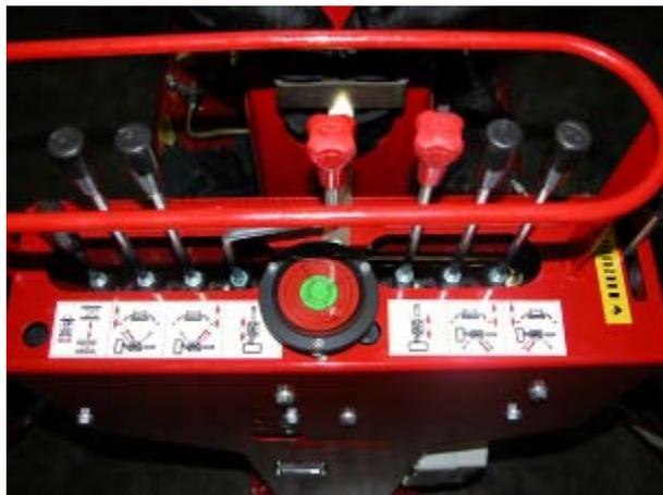
Before lifting the machines, the operator has to choose the working load through the 120/200kg selector, located on the control panel.
