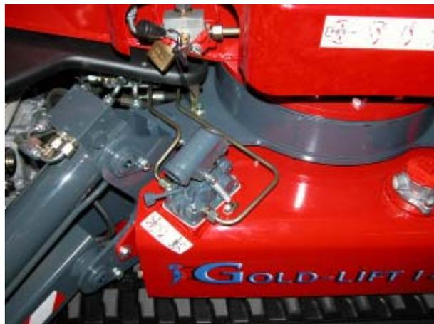
In order to move the basket, you need to pump the oil manually and at the same time to use the controls for the arms movements located on the undercarriage.
