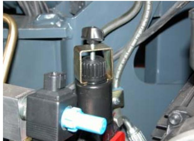
As soon as the emergency operations have been completed, don't forget to remove the mechanical commutator of the deviator and to restore the standard configuration of the deviator. The presence of the mechanical commutator of the deviator during the work jeopardizes the safety of the machine, causing possible dangerous situations.
