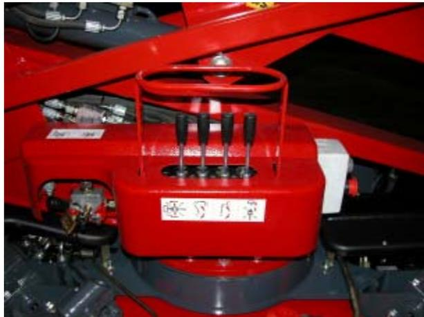
It is possible to move the aerial part only if the machine is stabilized and levelled (max 1°). This condition is signalled by the 4 flashing lamps that are on, when the outriggers lay on the ground and the machine is lifted.
