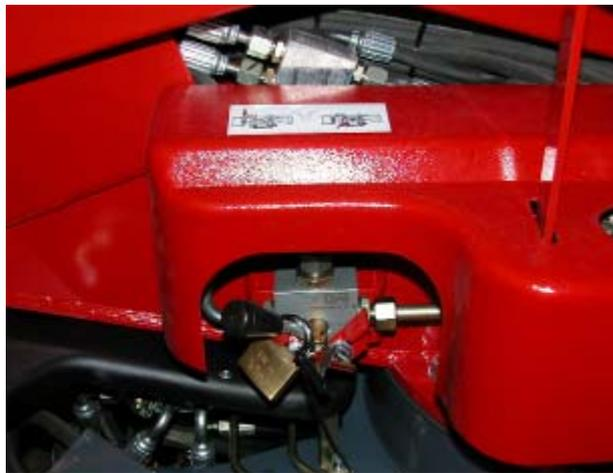
NOTE: in the model 1470, when you are using the emergency descend, the jib cylinder cannot be activated, then when the arm is completely down, the basket is at about 1,8 m height. In this case, in order to help the operator, you have to use an external tool (for example a ladder).
