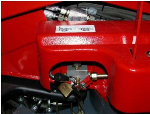
The valveblocks convey the oil to the cylinders that move the machine. The setting of the machine speeds is made by registers at the sides of the valveblock, that limit the spools' run bypassing some of the oil to the tank. Such settings cannot be altered, since the speed of the machine is set by law.
