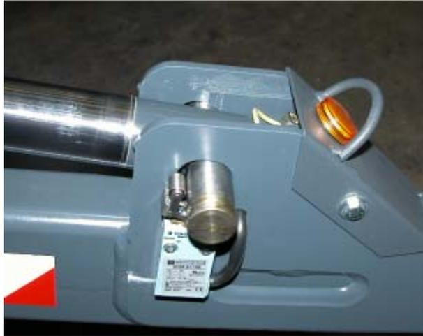
When all 4 outriggers send the signal to the electric panel, the machine is stabilized and a lamp lights on the electric panel (lamp outriggers on the ground).
