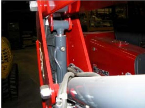
The oil pushed by the first cylinder is sent to the second cylinder located under the basket. This is equipped with a double block valve and two anti-shock valves, to get rid of the overpressures due to an improper basket levelling.
