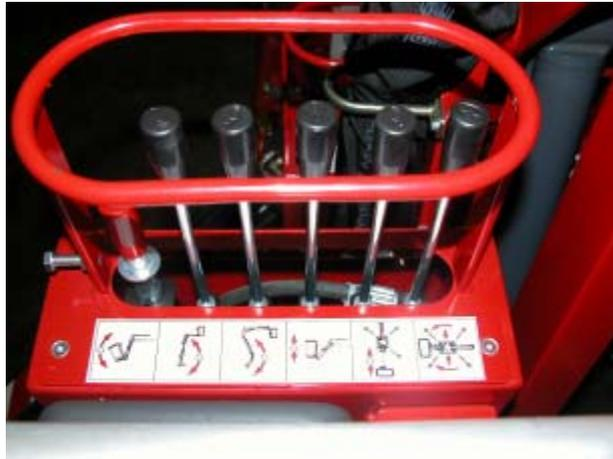
There is also the possibility IN EMERGENCY SITUATIONS, to control the aerial part from the ground through the valve-block located on the turret.
