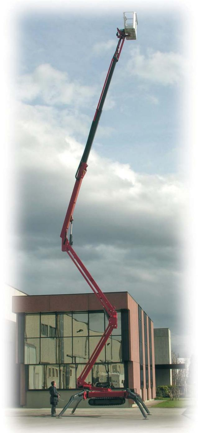
The new remote control also allows return movements to be performed in the event of a loss of stability.
